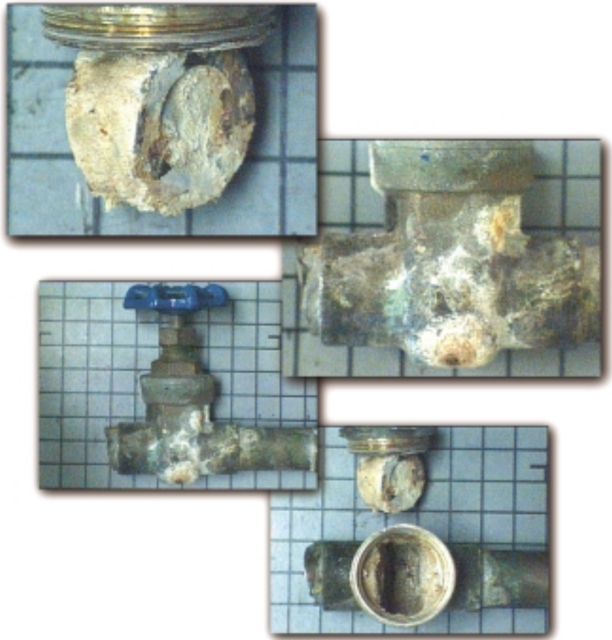
Figure 1. Typical examples of valves that have been dezincified
