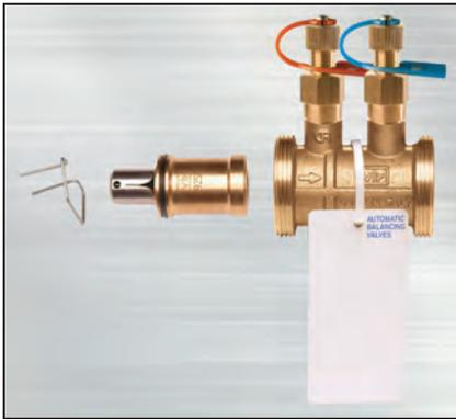
Insert the fixed housing end of the cartridge into the valve body in the direction of the flow arrow and press fully into position.
