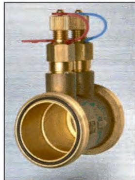
After the pipe connectors and union nuts have been fitted to the pipe, the valve body may be assembled. Ensure that the body o-rings are in place and that the arrow on the body is in the same direction as the flow. Hand tighten the union nuts to the body, making sure the valve body and pipework are in line. Using a correctly fitting wrench or spanner, further tighten the union nut ¼ turn. Excessive force is not required.
