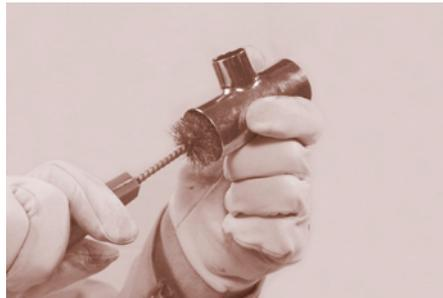
Figure 3. Reaming: Deburring Tool
